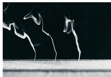
▲ Fig.1: Oil thread test to EN 1822-4 for testing testing EPA, HEPA and ULPA filters for leakage
