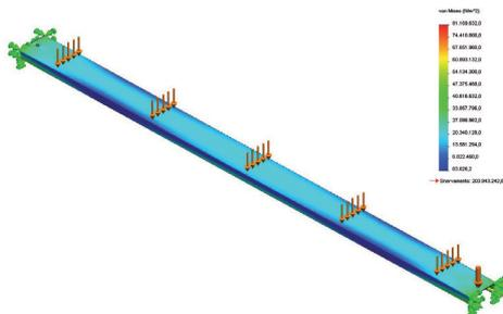
Structural inspection with load of 400 kg/m<sup>2</sup>
