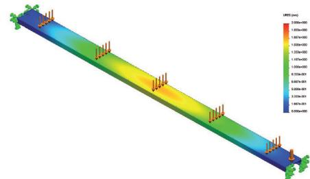
Check for deformation with 400 kg / m<sup>2</sup>
